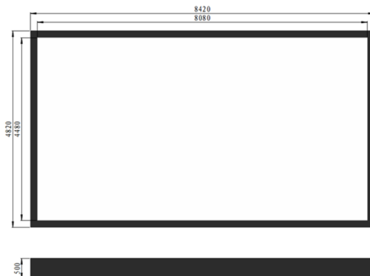
Figure 2-11 Dimensions for Protective Perimeter Wall Zone
